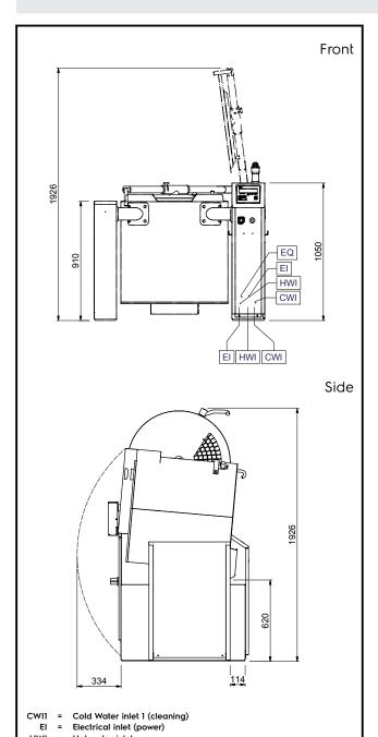
**Electric** Supply voltage: 400 V/3N ph/50-60 Hz Electrical power max: 31.5 kW Installation: Distance back floor tilted: 620 mm **Key Information:** 30 °C Working Temperature MIN: Working Temperature MAX: 121 °C Vessel (round) diameter: 695 mm Vessel (round) depth: 500 mm External dimensions, Width: 1300 mm 1070 mm External dimensions, Depth: 1050 mm External dimensions, Height: Net vessel useful capacity: 150 lt Tilling mechanism: Automatic
